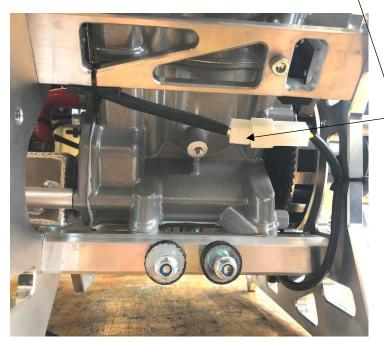
Take the longer side and connect it to the new installed stator.
