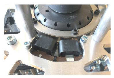
Use the 2 supplied screws and nuts to fixate the stator.
