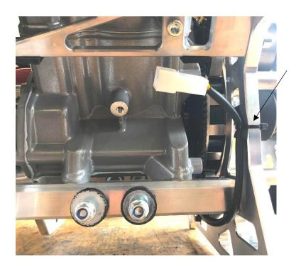
Place the stator cable around the engine mount as shown. Use a tie-wrap and fixate it as shown.
