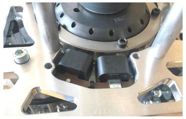
Next install the generator stator from the back side of the plate. Ensure the feeler gauge is fully between the stator and the magnets.
