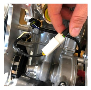
Place the short side of the connection cable between the front plate and the motor and connect it with the original stator.
