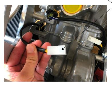
Next disconnect the original stator from the electrical wire harness.
