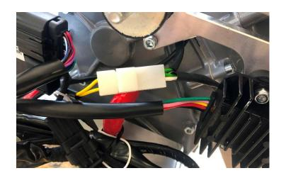
Finally connect the connection cable to the electrical wire harness.
