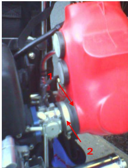
◆ **Note:** the carburettor socket is asymmetrical and can be turned so that the best possible position for maximum leg clearance can be achieved.
