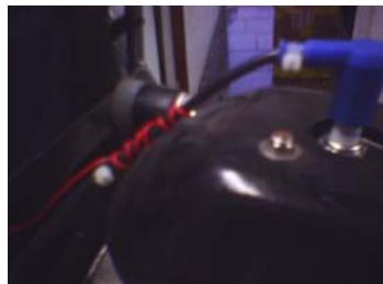
Wind at least three turns of the inductive cable between the ignition coil and spark plug connector and secure it with a cable tie on the ignition cable.
