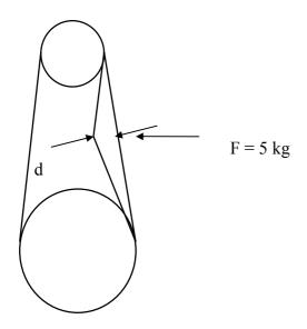
The belt should not move by more than 2 mm if a pressure of 5 kg is applied.
